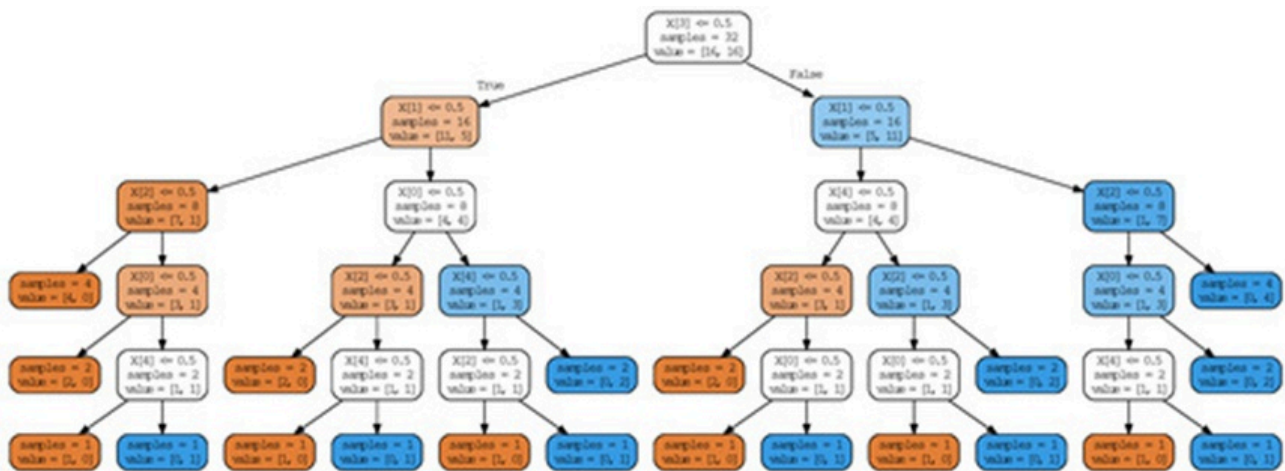
Figure 3. A diagnostic example highlighting how an intuitive classification rule generates an unwieldy decision tree graph. The mathematically ideal rule for this condition is \text{AtLeast3}(f_0, \dots, f_4) , but the standard decision tree trained to mimic this data expands to 19 decision splits, sacrificing human scannability.
