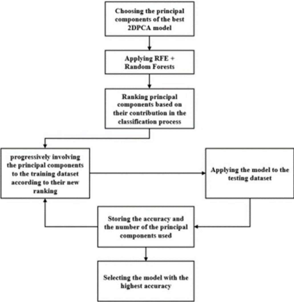
Figure 10. Flowchart of the combination process of 2DPCA and Random Forest in conjunction with RFE.
